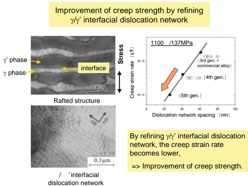
If the temperature capability is improved by 50°C (from 1100 to 1150°C), the cooling air inside the turbine blades, for example, can be reduced to improve thermal efficiency and thus the specific fuel consumption. The 50°C improvement corresponds to the improvement of about 6 times longer creep rupture life, provided that the alloy is used at the same condition. Subsequently, in this way the reliability of the parts will also be much improved.
