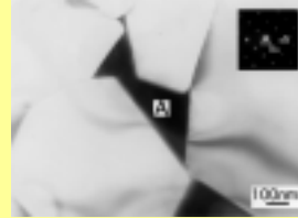
Crystallized grain boundary of \text{Lu}_2\text{O}_3 -doped \text{Si}_3\text{N}_4 ceramics
