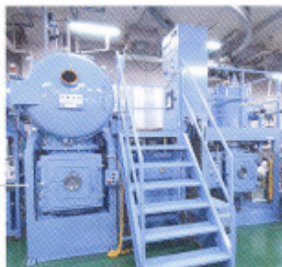
一方向/単結晶凝固炉 Directionally solidified / Single crystal casting furnace
