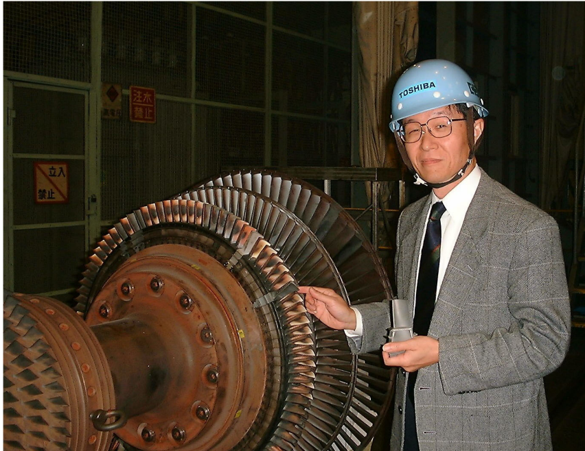
A 15MW-class turbine rotor installed TMS-75 blades.
