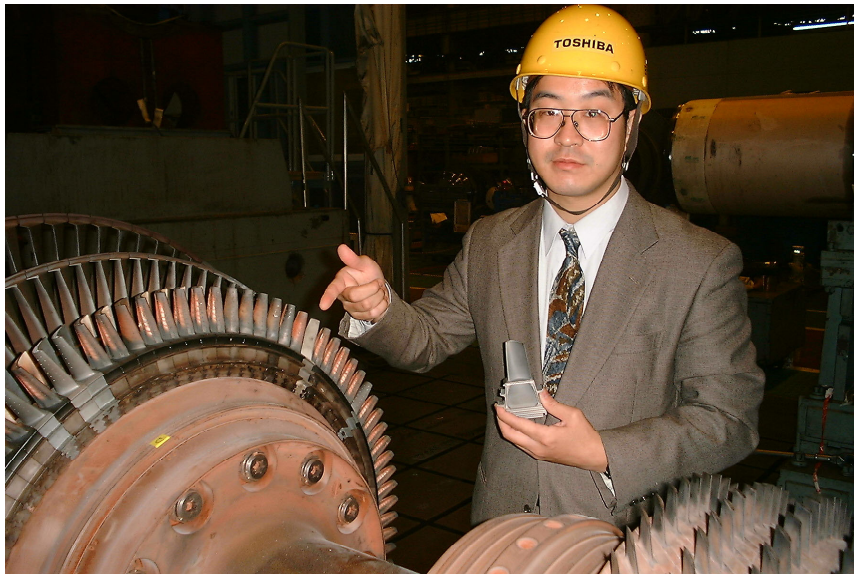
A 15MW turbine rotor installed TMS-82+ blades.
