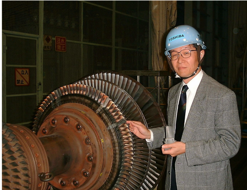
A 15MW-class turbine rotor installed TMS-75 blades.
